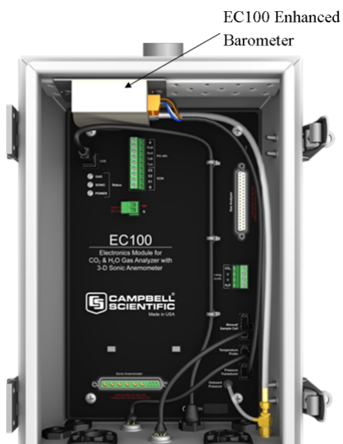
FIGURE A-2. Location of EC100 enhanced barometer
